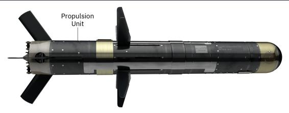
Javelin, a medium range "fire-and-forget" missile used by the U.S. Army and U.S. Marine Corps, is effective against tanks, bunkers, buildings, small boats, and armored vehicles. Aerojet Rocketdyne is the sole producer of Javelin's propulsion, which includes an integrated pulse motor with a launcher eject motor and flight motor in a single unit.
