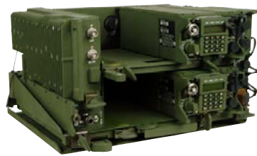
RT-1523 in a VAA mount, vehicular 50 W long range/short range
