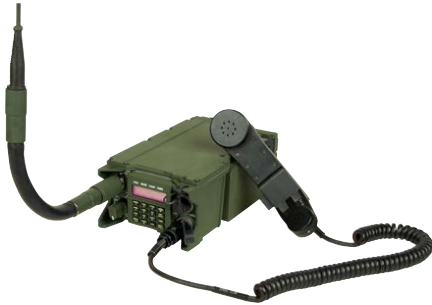
RT-1523 5 W manpack dismount configuration
