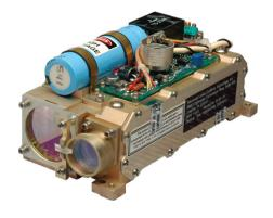
The ELRF-2 Flash-Lamp Eye-Safe Laser Range Finder is a Class 1 eye-safe, long-range laser range finder with an APD receiver suitable for a wide range of applications. With options such as lower beam divergence for smaller targets or increased range resolution for higher accuracy, the ELRF-2 can be configured for a specific application. The modularity of the unit along with L3Harris' engineering customization capability allows the ELRF-2 to be fitted to specific customer requirements.
