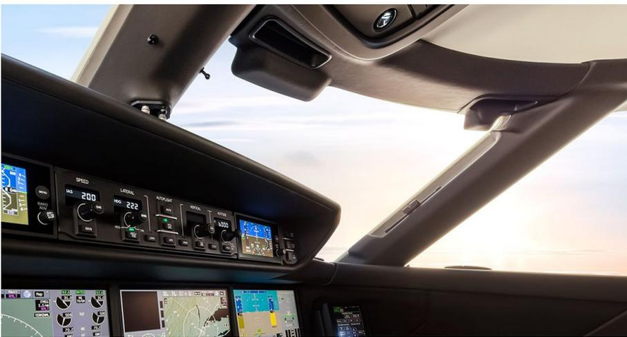
The ESIS-5000 Electronic Standby Instrument System is designed specifically for business aviation pilots as an agile and dependable solution. The intuitive panel-mounted, solid-state instrument provides the attitude, altitude, airspeed, heading, navigation and flight guidance information through an LED back-lit LCD touchscreen interface. The ESIS-5000's space-saving footprint, easy installation, and complete digital design makes it the ideal standby for any aircraft operator.
