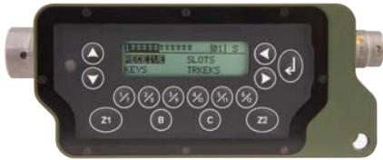
The small, lightweight, rugged TKL features instant-on start-up and a simplified key fill process, requiring just the push of a single button. Engineered for gloved-hand operation, this small and lightweight solution is ruggedized to withstand demanding conditions faced by forward-deployed teams.
