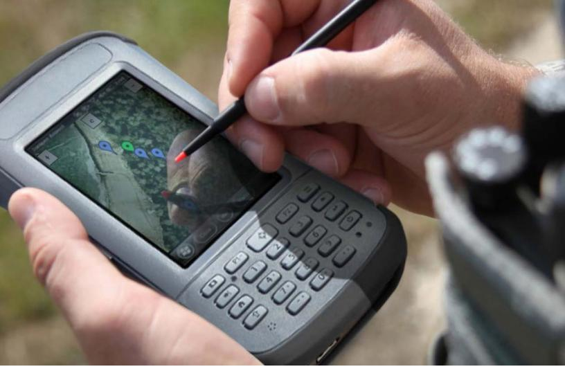
The RO-MAP is a software application that runs on a personal data assistant (PDA) or smartphone and provides vital situational awareness (SA) information quickly and reliably. It utilizes the functionality of a PDA along with the beyond line-of- sight (BLOS) capability of the RO tactical radio to provide a common operating picture (COP).
