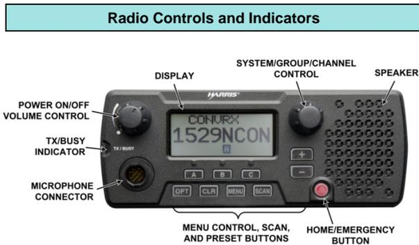
Figure 1: XG-25M Mobile Radio (Front View)
