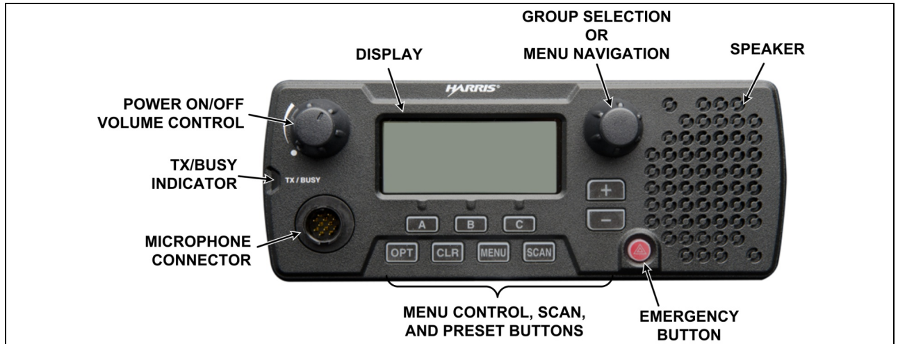
Figure 10-1: CH-25 Front Panel Components
