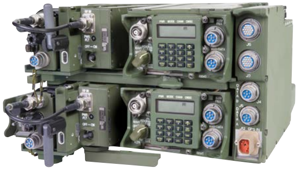
Dual RF-330UL-V125 mounted within an AN/VRC-92 radio system
