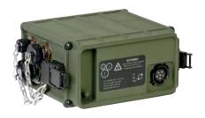
The RF-5910-PS005 Power Supply provides a regulated output voltage to the AN/PRC-117G(V)1(C) and RF-7800M-MP FALCON III® Manpack transceivers from an AC input range of 85-265 VAC/47-440 Hz and a DC input range from 10.5 to 34.5 VDC. It is designed to supply power to the Falcon III Manpacks, without performance degradation, through a TX-RX frequency range from 30 MHz to 2 GHz.
