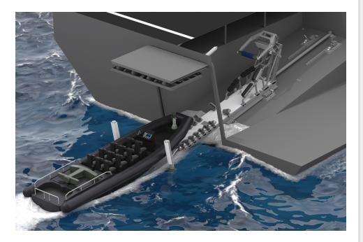
The system is placed at the stern of the main vessel for a fast and safe launch or recovery.
