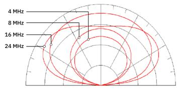
RF-1944-Series Broadband Inverted VEE HF Antenna © 2020 L3Harris Technologies, Inc. | 04/2020 SP149
