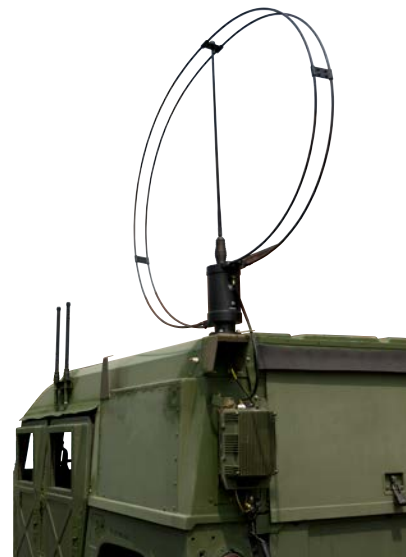
RF-3134-AT003/5 mounted on vehicle
