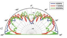
RF-3165 Typical Radiation Pattern when mounted on the Falcon III manpack over ground
