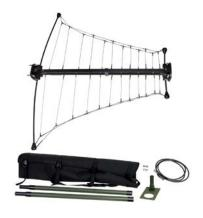
The RF-3192C-AT422 is a transportable wideband directional Log Periodic Antenna (LPA) covering the frequency band from 225 MHz to 450 MHz. It is optimized for high gain to extend the range of wideband networking waveforms, such as ANW2, SRW, and WNW.
