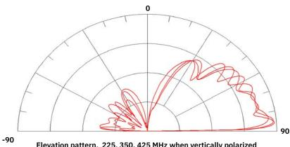
Elevation pattern, 225, 350, 425 MHz when vertically polarized over real ground
