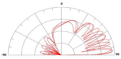
Azimuth pattern at 5° above horizon
