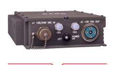
The RF-5055PS is a low-profile solution providing a regulated 26.4 volts DC at 18 amps. The power supply is designed for use with the RF-5833H-PA 150-watt Power Amplifier in tactical installations with duty cycles up to 20%. When paired with the RF-5056PS DC/DC converter, the RF-5055PS supplies available AC power to the auxiliary input of the DC/DC converter to conserve vehicular battery life. The RF-5055PS may be mounted on the RF-5071VSM-03 shock mount for use in harsh environments.
