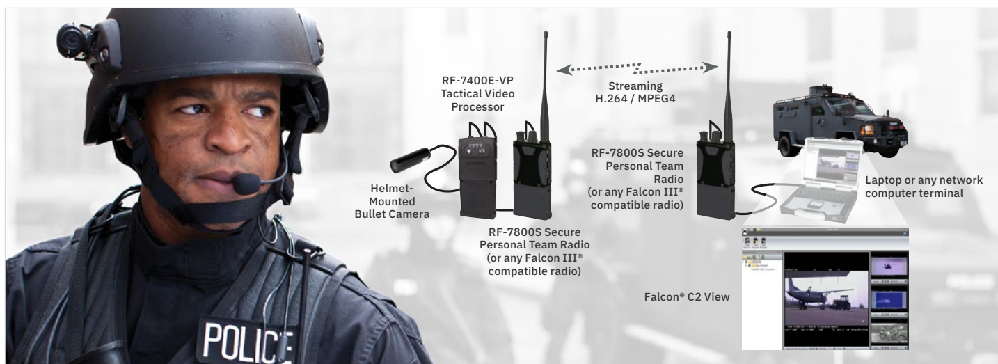
Operation concept for helmet-worn scenario: TVP acquires and shares short-range surveillance footage from helmet-mounted camera
