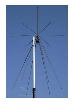
Engineered for on-the-move tactical missions, the L3Harris RF-9072-AT00X is made with composite materials that ensure low weight and superior resistance against atmospheric interference. This portable, wideband, disc-cone antenna is robust enough for stationary use with rapid, user-friendly setup. Composed of a support head with a built-in line transformer, the RF-9072-AT00X includes six disc elements, and six cone elements which are divided into two sections.
