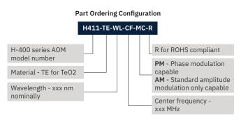
H411-TE-532-80-AM-R is the standard configuration. Please call the factory for additional configurations. Requires H-400 AOMseries compatible driver and cable. Specifications subject to change without notice.
