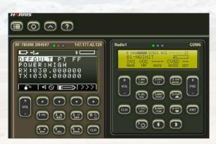
The L3Harris Soft KDU provides C2 operators remote access to radios from the hC2 interface.
