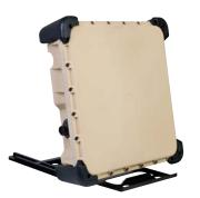
This L3Harris Land Portable BGAN Terminal features a system of manually pointed antennas engineered for military applications but is also appropriate for rapid deployment by law enforcement, homeland security or disaster-relief operations. When used with the L3Harris Falcon III® AN/PRC-117G(V)1(C) or RF-7800M-MP manpacks, the terminal allows networking capabilities to automatically route between mobile wideband LOS and Beyond-Line-Of-Sight communication nodes.
