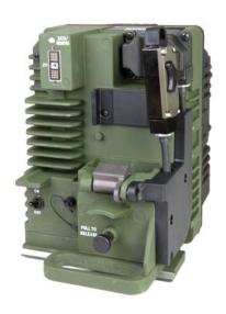
This VHF power amplifier covers the 30 to 108 MHz frequency, supplying up to a full 50 watts of forward power under demanding Voltage Standing Wave Ratio conditions. It also delivers excellent collocation performance in both fixed frequency and frequency hopping modes.
