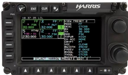
Optimized for use with the L3Harris Falcon III® RF-7850A-MR Multi-channel Airborne Radio, the RCU is airborne certified for in-cockpit integration. It is ideal for aircraft retrofits or when building entirely new systems. The unit features a full-color, NVIS-compatible graphical LCD screen with a familiar aviator radio control interface. User-friendly navigation menus, soft key selection and preset upload capabilities help simplify even the most complex airborne missions.
