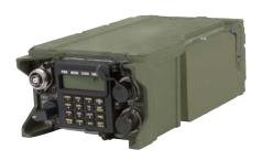
The RT-1702 rapidly adapts to changing mission needs. When deployed as a manpack by dismount soldiers, the radio uses a standard Point-To-Point interface to allow Command and Control applications to access tactical networks. The L3Harris Vehicular Amplifier Adapter supports mobile use and networked
