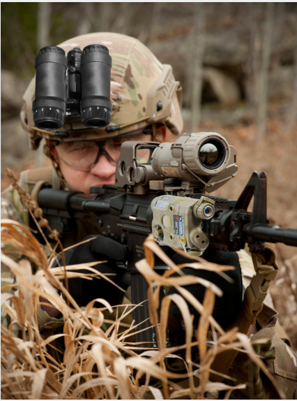
Integrated infrared and visible aiming lasers
