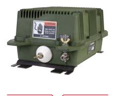
The RF-5382H automatically matches the output of the Falcon II® and Falcon III® series of HF transceivers to a variety of whip, dipole and long-wire antennas over the 1.6 to 30 MHz frequency range. The coupler's tuning time from memory is less than 150 milliseconds, supporting advanced waveforms and network protocols requiring rapid, reliable frequency changes in severe environmental conditions.
