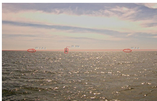
Figure 2 -Image (video) based obstacle tracking and classification
