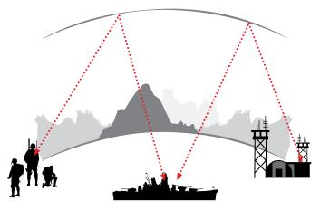
Adjusting HF frequency and antenna orientation enables radio waves to either traverse the ground (ground or surface wave) or refract off the ionosphere (sky wave).
