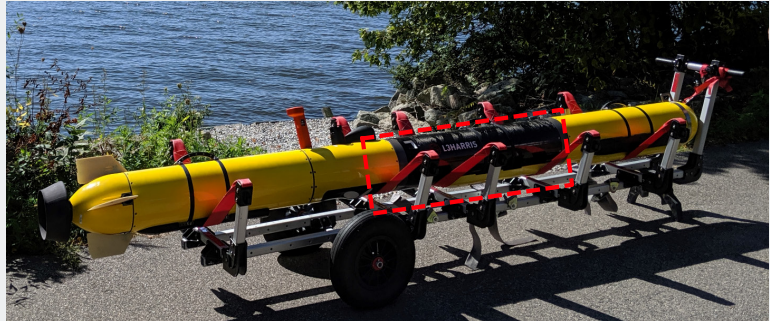
Figure 1 - Energy Module Integrated on L3Harris' Iver4 900 Unmanned Underwater Vehicle
