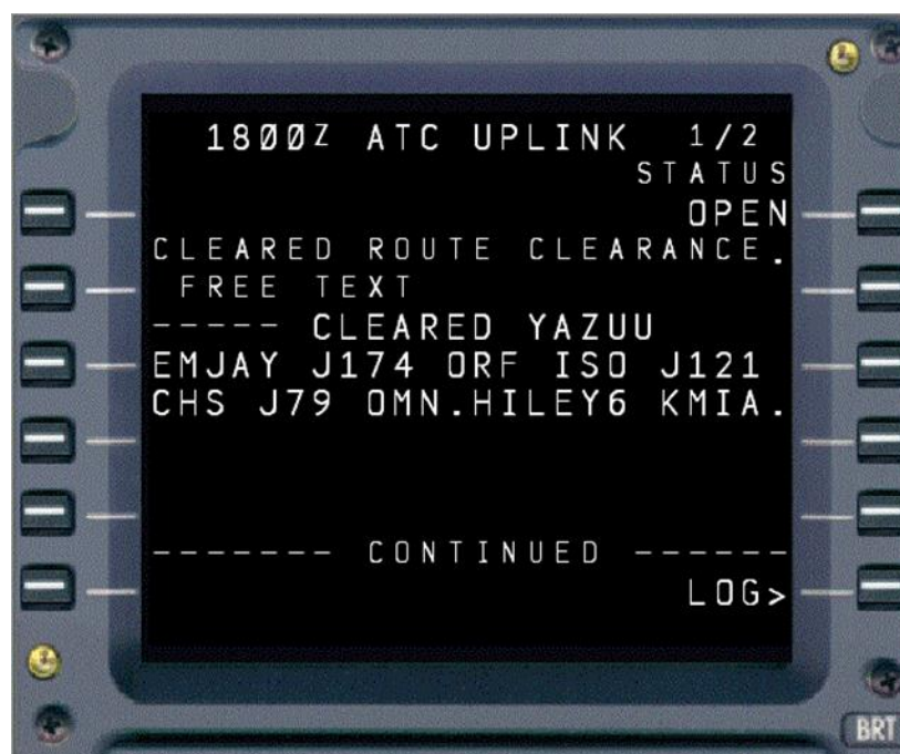
Figure 24. UM80 Full Route Clearance and Supplementary Route Free Text (B737 MCDU Test Bench – FAA Tech Center)
