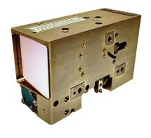
The CPHAR is L3Harris' next generation of low-cost mature diode-pumped laser range finders sized at 2.1 inches x 3.1 inches x 5.1 inches, weighing less than 2.0 lb and consuming less than 35 W. Designed for ground vehicle applications that support repetition rates up to 5 hertz with extended standoff ranges.
