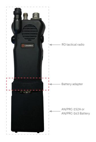
AN/PRC-152A battery = 33 rechargeable RCR123A batteries
