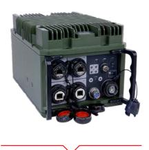
The L3Harris RF-7800W-IU30X Network Interface Unit (NIU) is a multi-port, Layer 2, Power over Ethernet switch. The NIU includes multiple DC outputs which allow it to power RF-7800W radios and accessories. The unit also supports wide-range input power, supporting deployment into a diverse set of operational environments. The NIU is MIL-STD-810G ruggedized and includes a SIP server and an autoredundant link for a seamless switch over to a second radio link if primary goes down.
