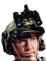
The MAVIS system can be used as a standalone day display or can be coupled with the AN/PVS-31/31A BNVD I2 platform for night operation.
