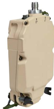
The L3Harris RF-7850D-MM00X is an attachable, software defined module that decisively expands the RF-7850D from a 2-channel radio to a multifunction 3-channel radio. The Mission Module provides seamless interoperability between forward deployed ground-based tactical units through wideband, crossbanded intel, linking three disparate networks together through a single all-informed Common Operational Picture.
