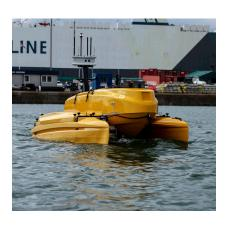
The C-Cat 3 Autonomous Surface Vehicle is a rapidly deployable catamaran ideally suited to shallow water operations in inshore and coastal environments.
