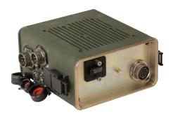
The RF-7914-PS001 can be used as an alternative to either the 20-Watt Vehicular Adapter Assembly or the radio battery box and MIL-STD manpack batteries.
