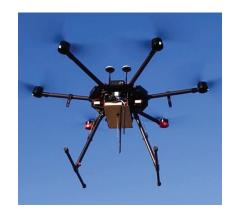
Rio Flex dual-channel SDR and small form factor processor mounted on a hexacopter for JICD precision geolocation applications
