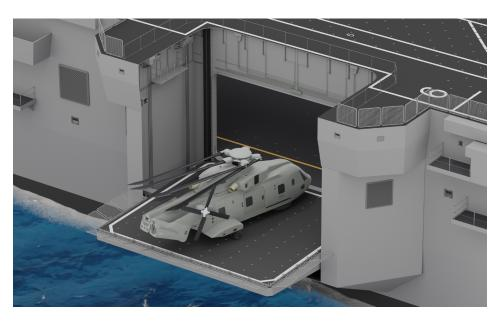
The elevators are shock-qualified. They can also be used to transport:
