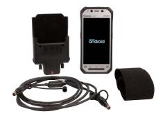
The RF-3577-95EN Rugged 4.7-inch Android Phone is designed for use by dismount soldiers. Software drivers required for L3Harris radio communications are pre-installed. The phone meets MIL-STD-810G certified for harsh weather conditions. Cables for radio data connection and charging are included.
