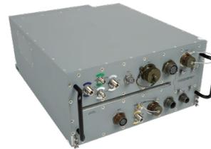
AN/ARQ-59 Electronic Frequency Converter (EFC) provides switching between the fore and aft RFAs
