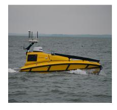
C-Worker 4 is a robust and capable Autonomous Surface Vehicle ideally suited to inshore and coastal survey
