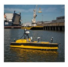
C-Worker 5 is an autonomous vehicle designed to support hydrographic survey work and to increase survey coverage in limited timeframes. A proven offshore survey "forcemultiplier", C-Worker 5 can operate for up to 8 days at a survey speed of around 5 knots.
