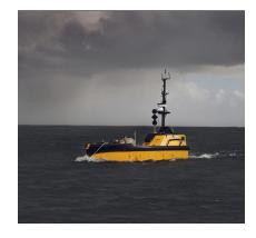
C-Worker 7 is a robust, offshore work-class Autonomous Surface Vehicle. Designed for inspection and positioning applications, C-Worker 7 can negate the need for a ship on station or seabed anchoring.
