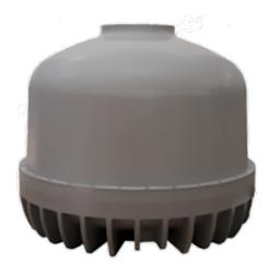
The NR-50 sensor is a pulse-compressed X-band transceiver. Transmission power can be selected by the user, from less than 1 watt (peak) up to 50 watts. The antenna is a slotted waveguide specially designed for navigation and surface applications. Its low weight and reduced dimensions allow for easy installation on submarine masts.
