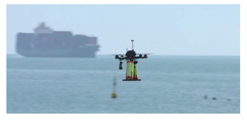
The software analyzes all images taken by a daylight camera and an infrared camera, looking for the MOB across the sea surface.
