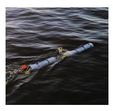
Iver is the first commercially developed family of low-cost autonomous underwater vehicles (AUVs). They are ideal for coastal applications such as sensor development, general survey work, sub-surface security, research and environmental monitoring. These modern AUVs are single man-portable and feature simple point-and-click mission planning.
