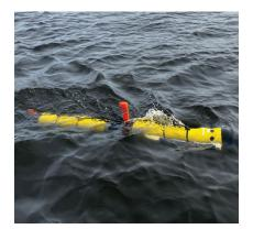
The Iver4 580 offers users a 300-meter depth survey system featuring hot-swappable battery sections that can be changed in the field without any special tools.
