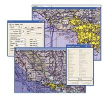
The LEGS Situation Display supports both geotiff and NGA Compressed ADRG maps. View JUs and tracks in user-defined Symbology based on MIL-STD-2525B with a map underlay. Hook tracks and obtain data readouts.
