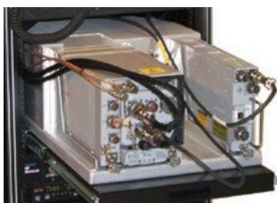
Rackmounted MIDS-LVT(1) cooling Tray with Terminal
